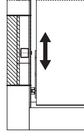
Fitting of the upper door end: When tighten the nut (Wrench 17) keep an even gap (4mm) between door and jamb
